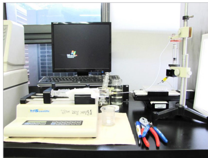
Fraction recovery system & XY Linear Positioners 추출시스템
